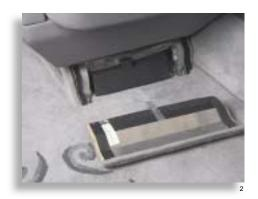
In and around the seat, 3M<sup>™</sup> Flame Resistant Scotchmate<sup>™</sup> Reclosable Hook and Loop Fasteners secure a kickplate/access panel, hold seat cushions in place, and fasten carpeting to the floor.
